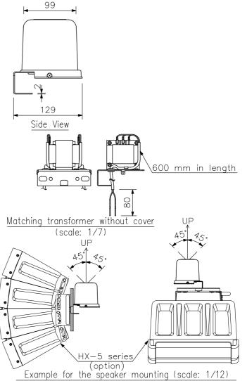
\* When installed outdoors, mount the MT-200 in either way that the tilt angle of its top surface is kept within 45° from the vertical axis. Exceeding this angle will deteriorate the speaker's water-resistant capability.
